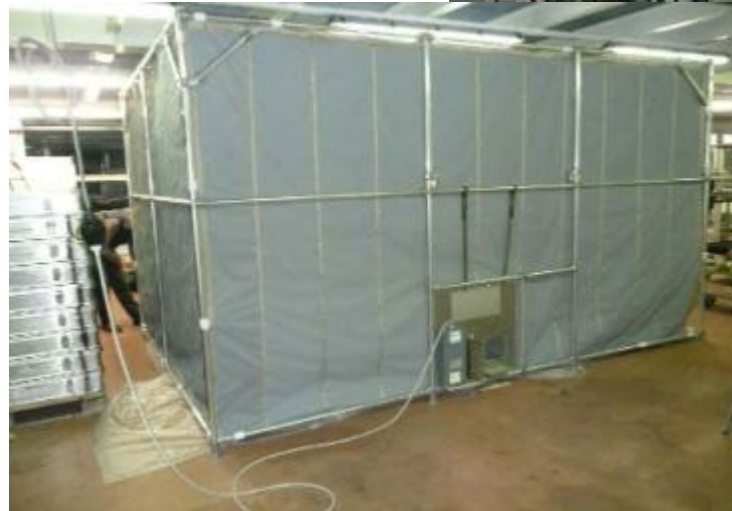
Shielded shelter structure
