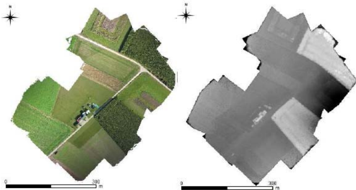
Figure 1. Orthomosaic (left) and Digital Elevation Model (right) based on imagery acquired from the TMPSYS-X8 UAV
